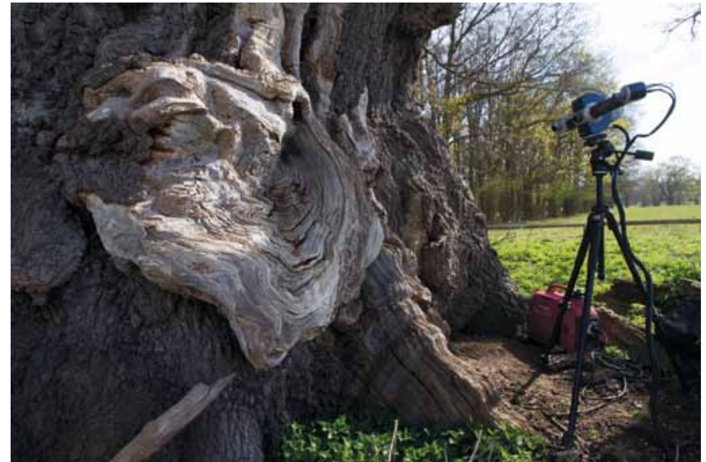
The signing Oak in Windsor Great Park being recorded with a Breuckmann 3D SmartSCAN.
