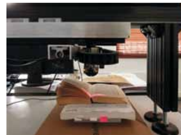
A Lucida Scanner that has been modified to work horizontally to record the pages of a book.
