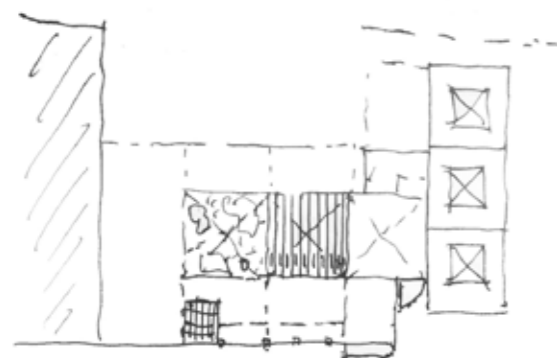
The new Research Lab is designed around a Silo-shaped void, 3 squares, each 10 x 10m
