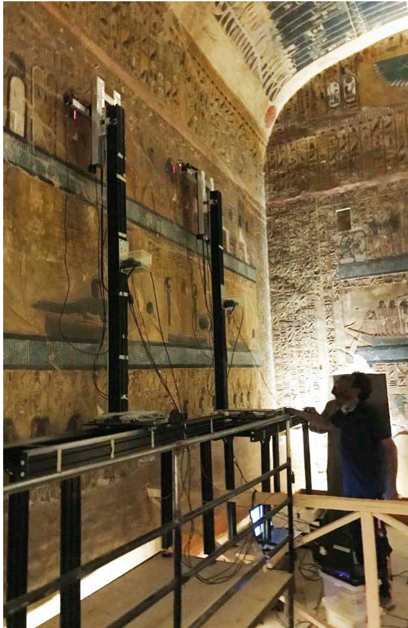
Scanning in the Sarcophagus Room with two Lucida 3D Scanners.
