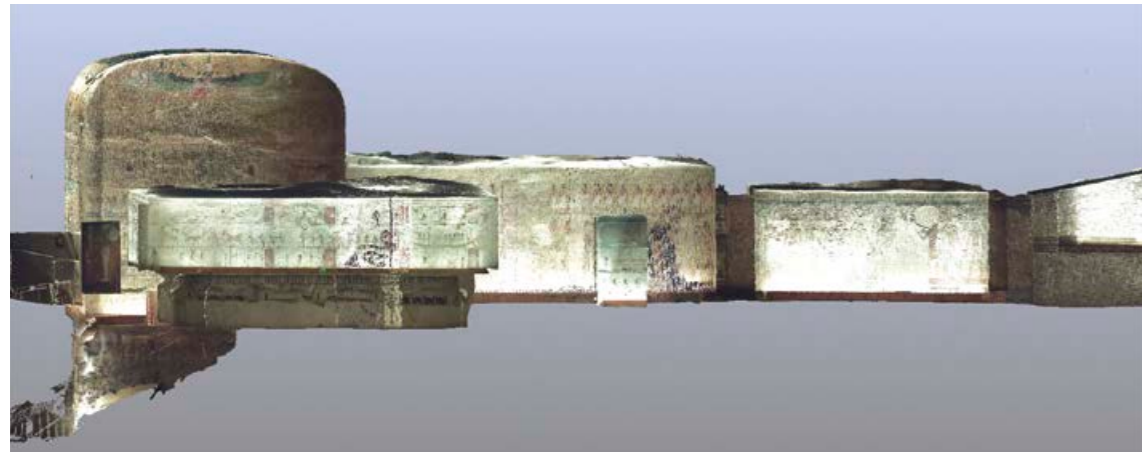
LiDAR data being processed in order to produce a walk-through model of the tomb.
