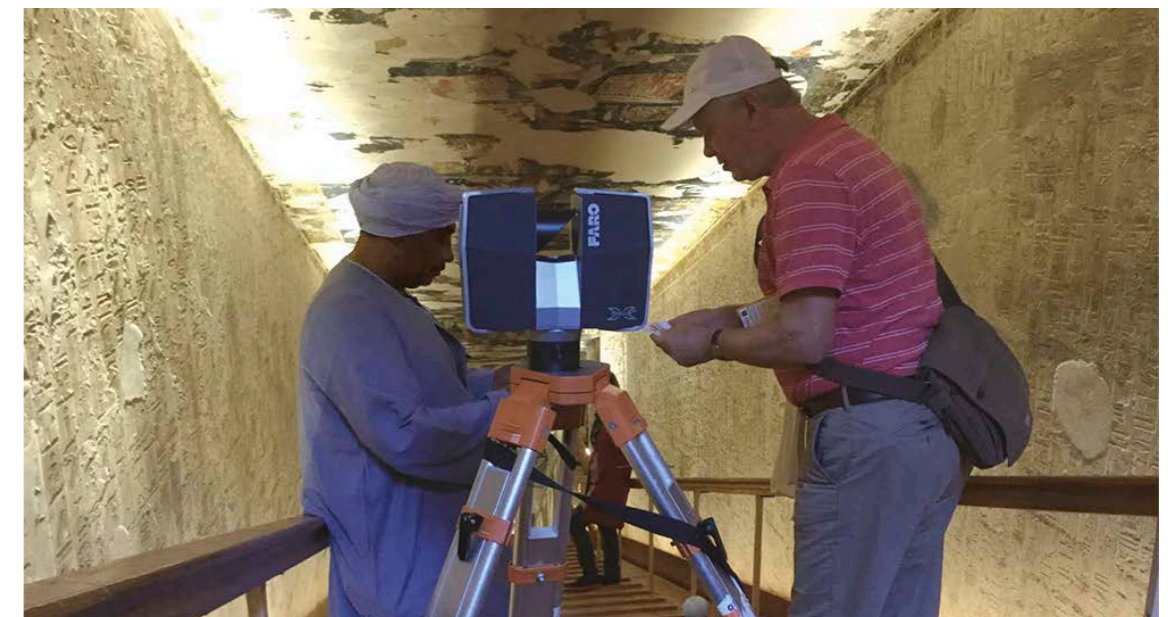
LiDAR scanner at the entrance to the tomb of Seti.
