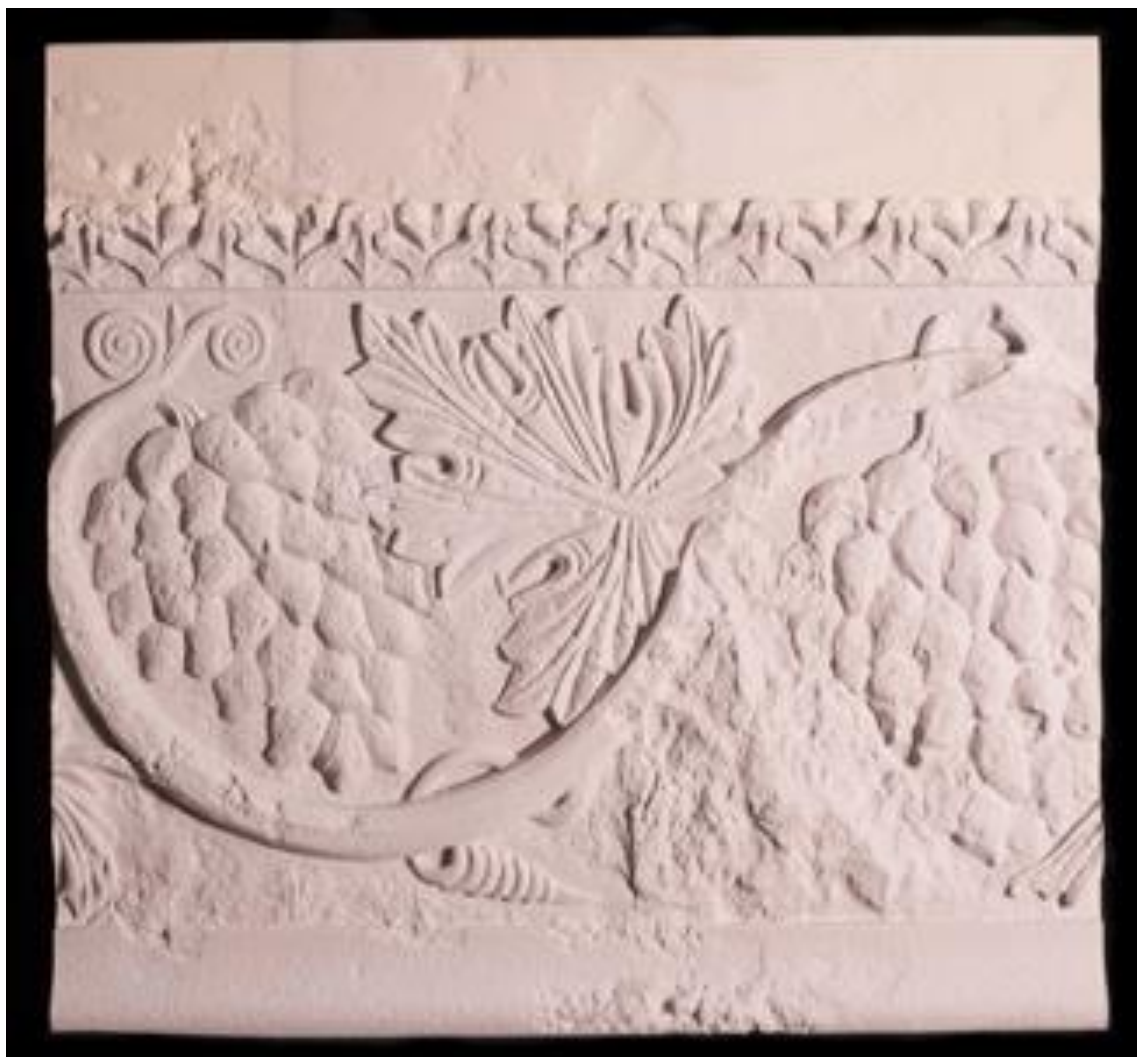
Image of the routed section of the arch of the Temple of Bel in Palmyra routed into high density polyurethane.
