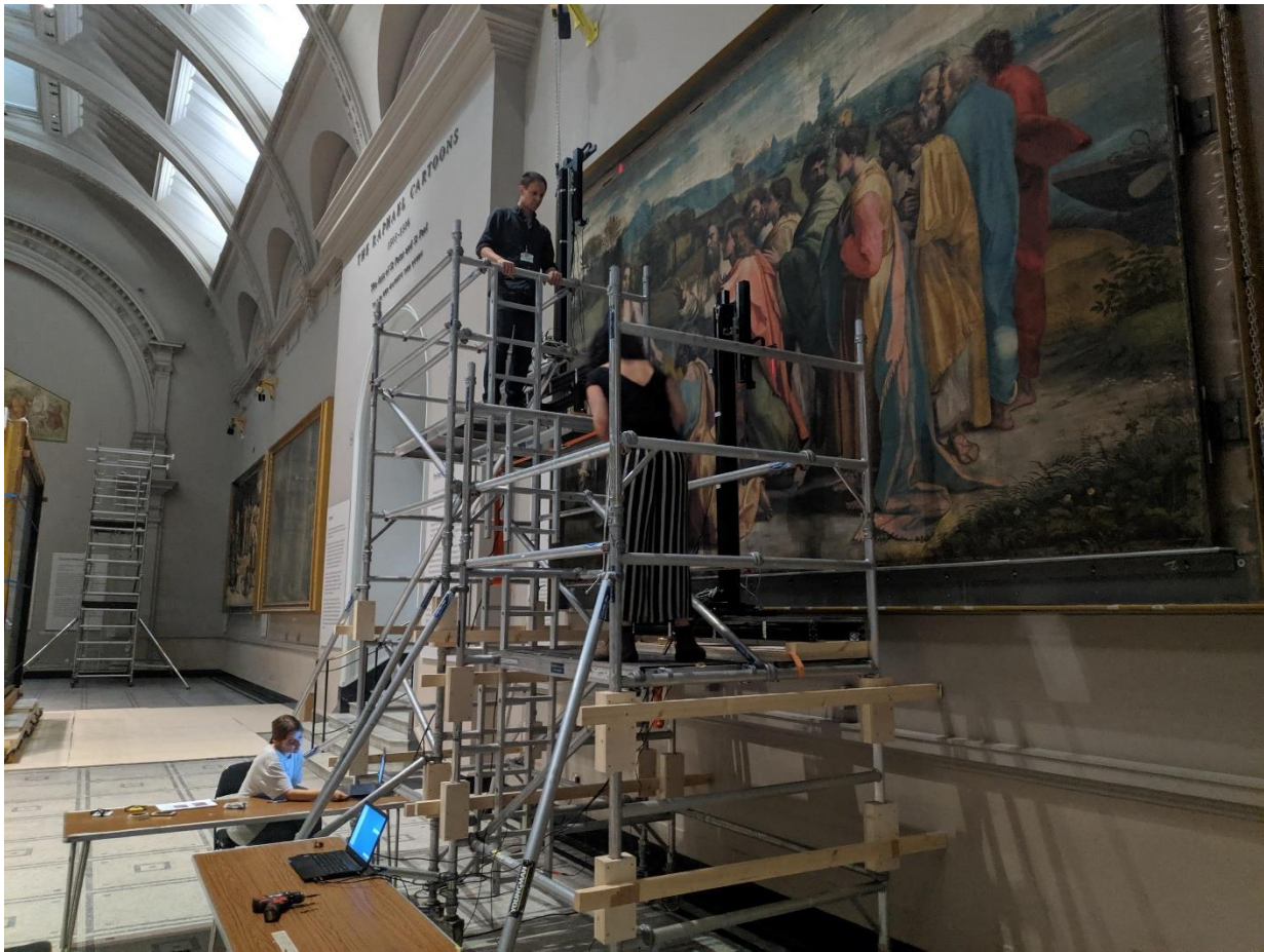
The Factum Foundation team using the Lucida 3D Scanner to record the surface of one of the Raphael Cartoons at the V&A. © Gabriel Scarpa for Factum Foundation
