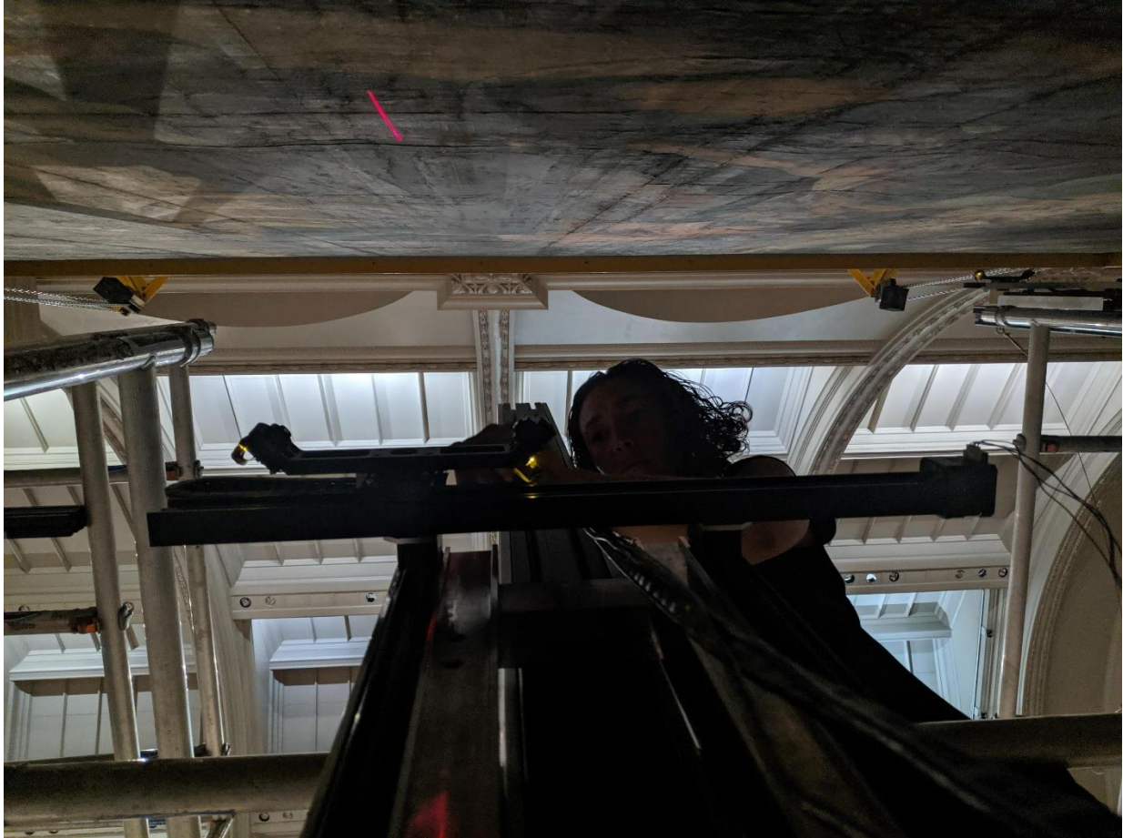
Detail of the Lucida 3D Scanner recording the surface of a Raphael Cartoon at the V&A. The technology operated by Factum Foundation is entirely non-contact and operates at safe distance from the artwork at all times.
