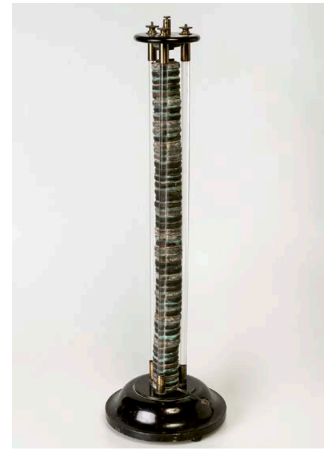
A voltaic pile, made by Apps, London 1860s.
