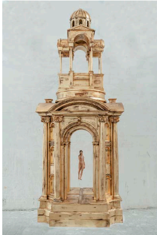
The original Tabernacle was damaged during the Civil War, losing its top half. For its recreation, Factum Foundation created a 3D model based on a historical picture, which was then split into several parts to be 3D printed or CNC-milled individually.
