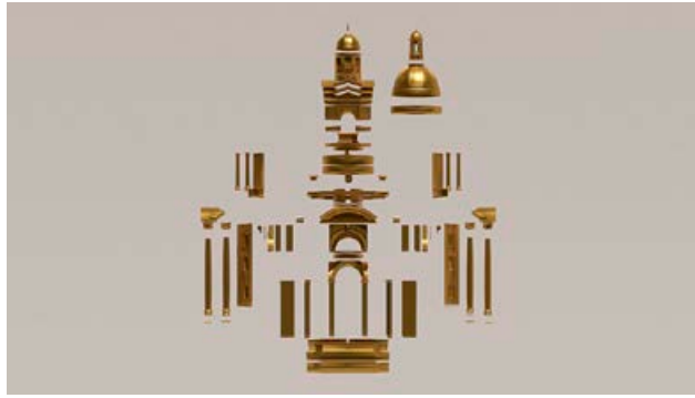
The original Tabernacle was damaged during the Civil War, losing its top half. For its recreation, Factum Foundation created a 3D model based on a historical picture, which was then split into several parts to be 3D printed or CNC-milled individually.
