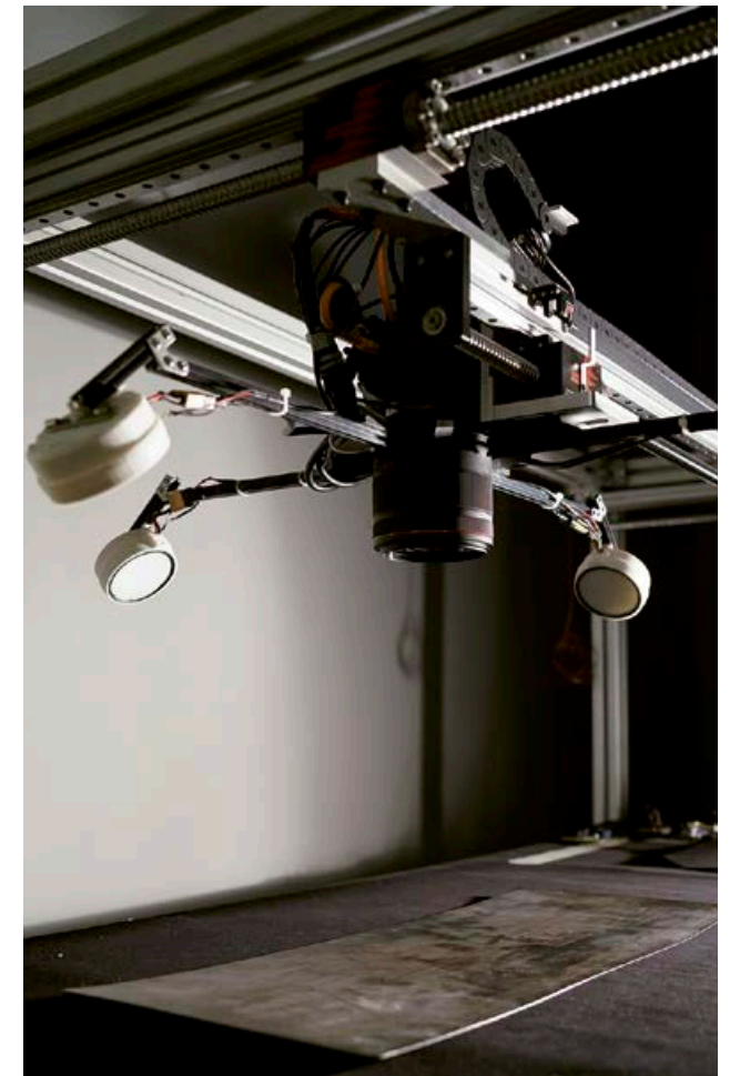
Selene Photometric Stereo System.
