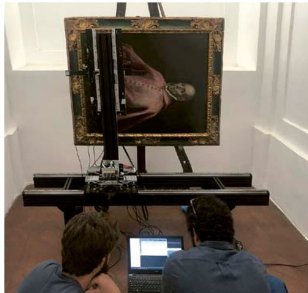
Recording the surface of the original Portrait of Cardinal Tavera by El Greco using the Lucida 3D Scanner.
