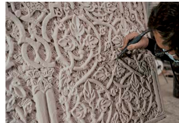
Retouching some of the finer details on a plaster cast yesería from Casa de Mesa.
