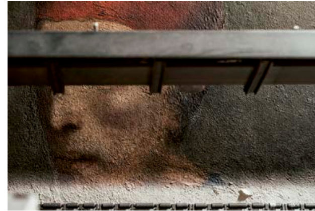
Printing the colour of Alonso Berruguete's Portrait of Cardinal Tavera over the textured surface created using elevated printing by Canon Production Printing.
