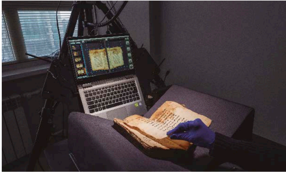
Portable Manuscript Scanner being used at the State Archives in Makhachkala, Dagestan to record their collection of Arabic manuscripts
