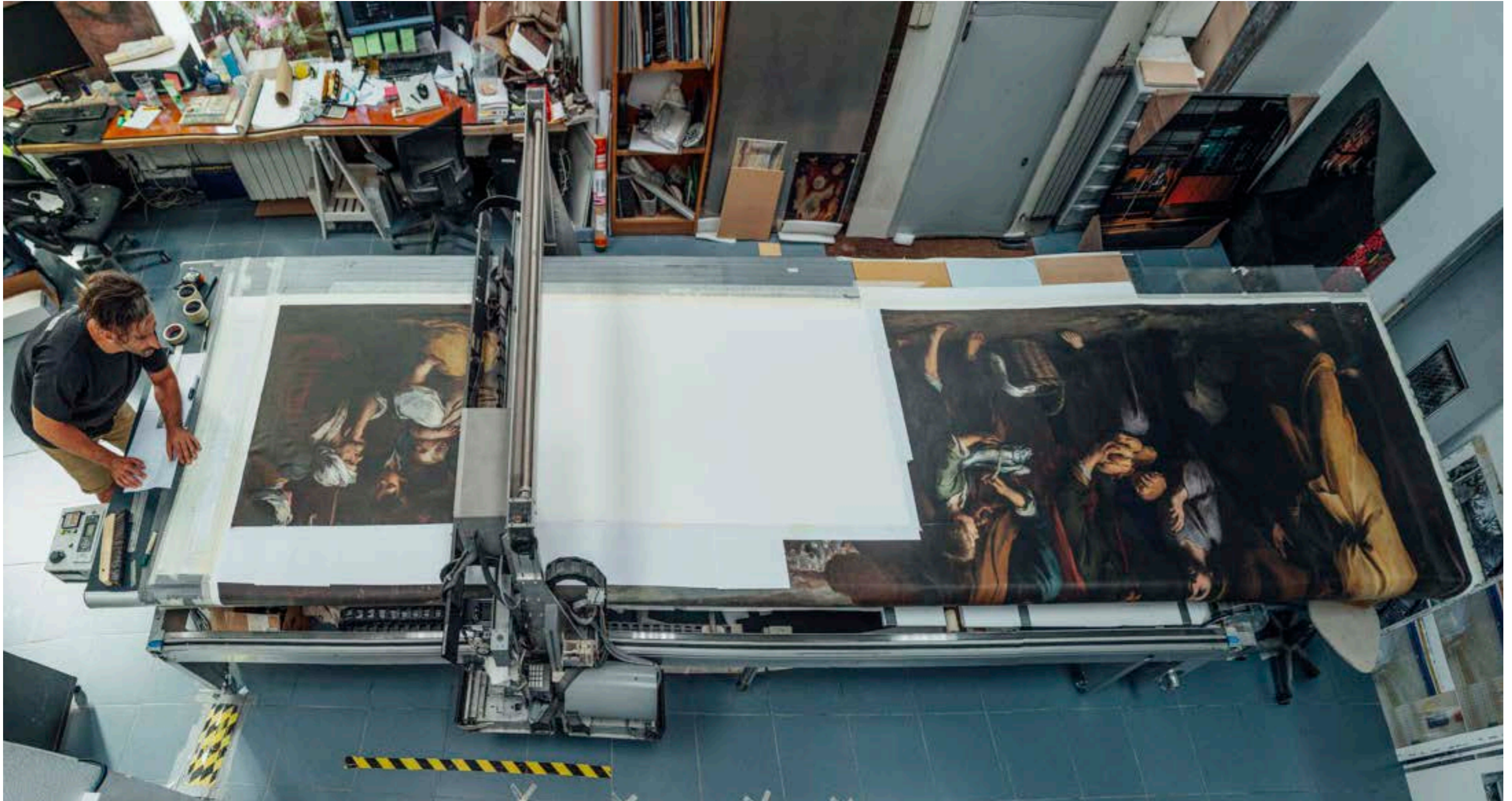
Printing the Bartolomé Esteban Murillo's The Miracle of the Fish and Bread with Factum's flatbed printer
