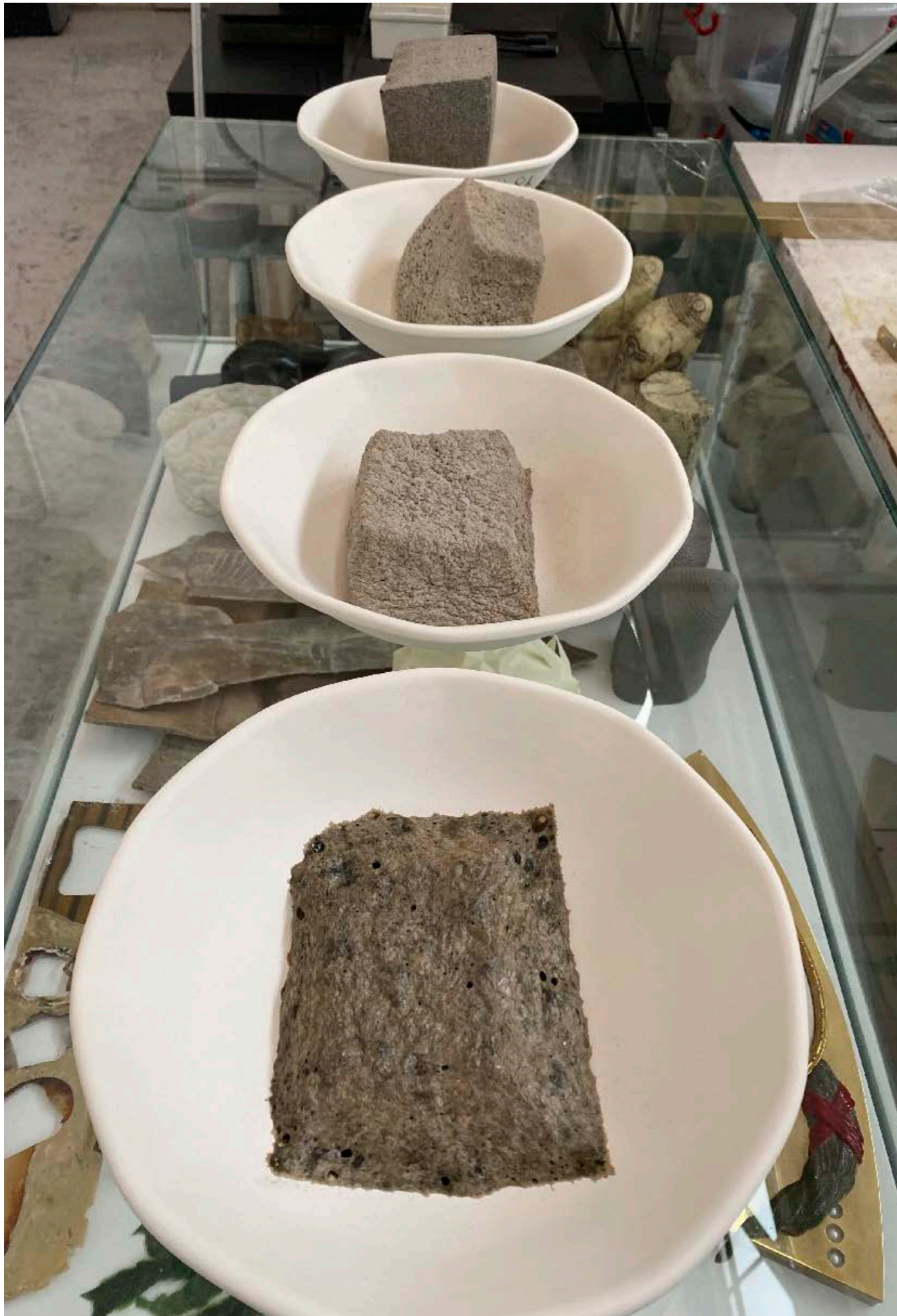
Experiments with Foamlas® heated to different temperatures
