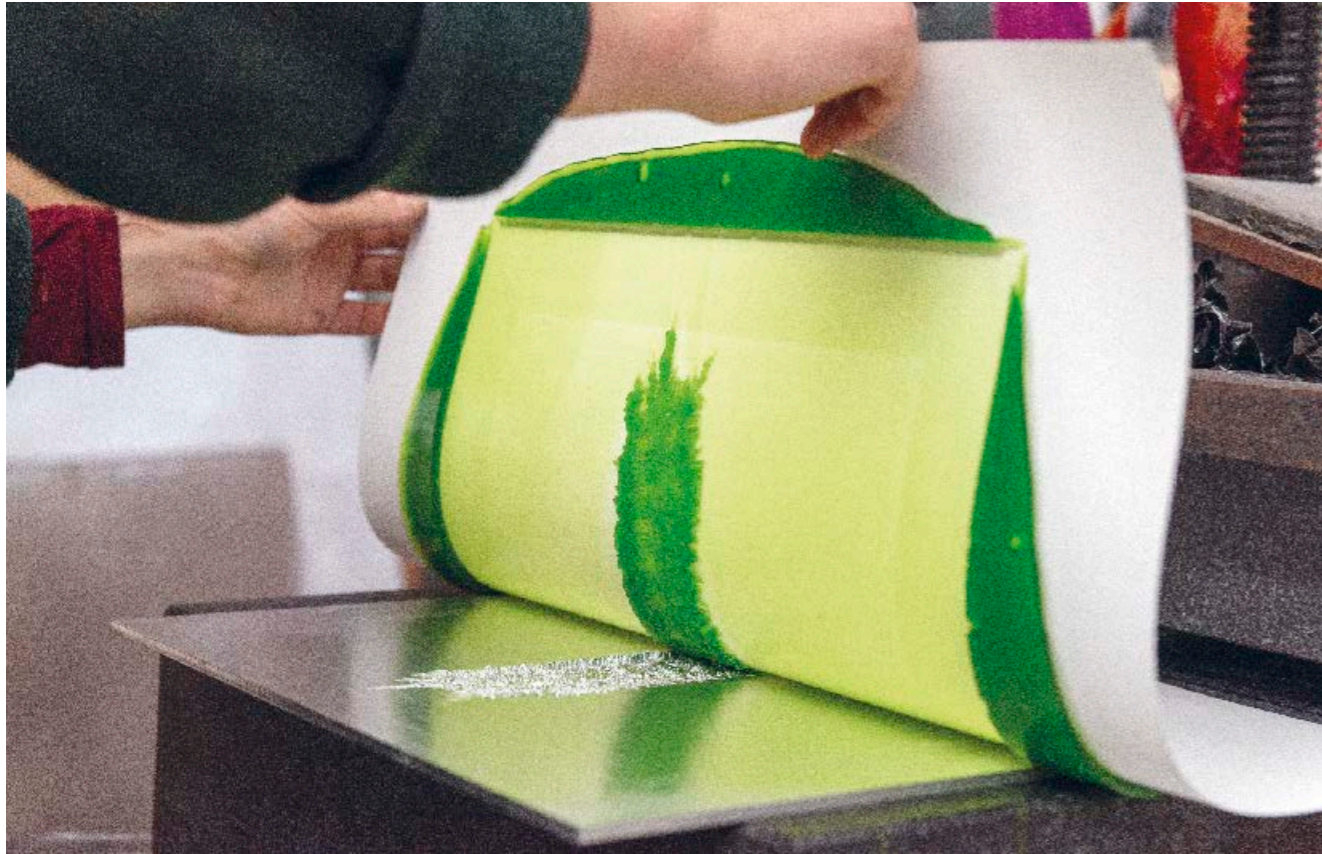
Woodburytype: Constanza Dessain printing a CNC-milled woodburytype plate in pigmented gelatin
