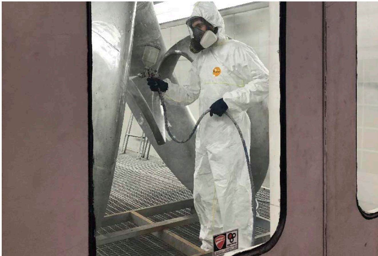
The workshop also contains a pressurised heated painting chamber for special paint finishes
