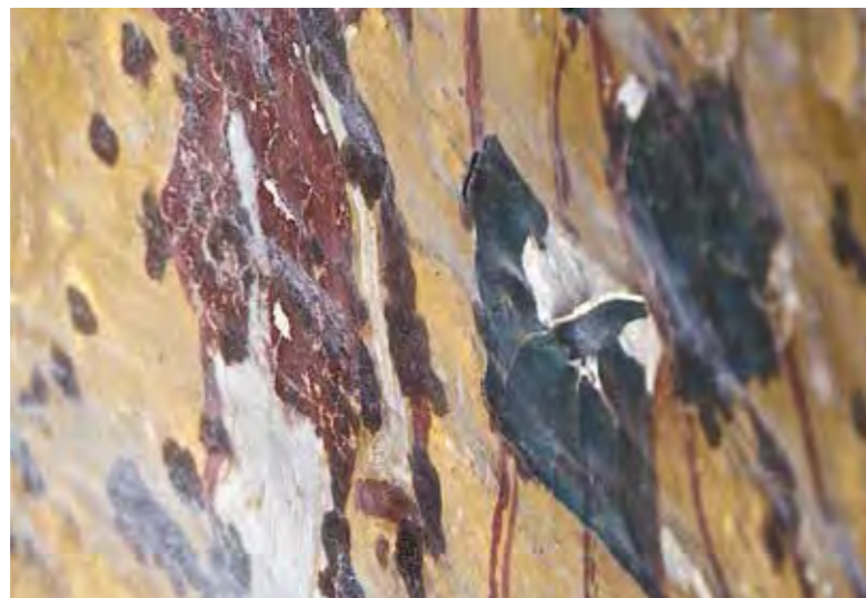
The surface of the East Wall in the burial chamber of Tutankhamun showing flaking paint and a sheen from surface painted Paraloid. Photo by G. Dupond, courtesy of Factum Arte.
