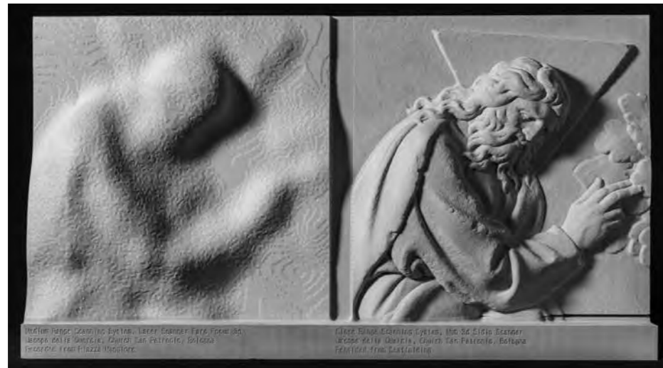
CNC milled data from a FARO Focus 3DX 330 LiDAR scanner (left image) and same section of the façade of the Church of San Petronio recorded with a Nub3D White Light scanner (right image). Both are milled at actual size.
