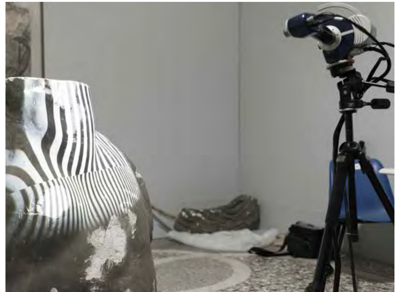
Breuckmann white light scanner in Palazzo Bonaguro recording a fragment of the Colossal Horse, 2017–2018.
