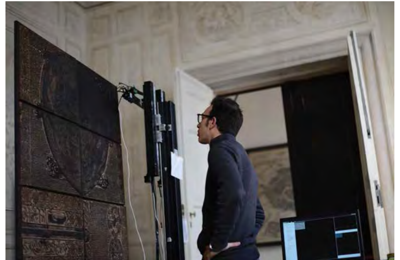
Mario Costa, student from the Master of Digital Architecture who have interned at ARCHiVe in Venice and Factum Foundation in Madrid, carrying out the 3D laser scanning of the cherry-wood printing blocks of the 16th-century "Mappa Turchesca".
