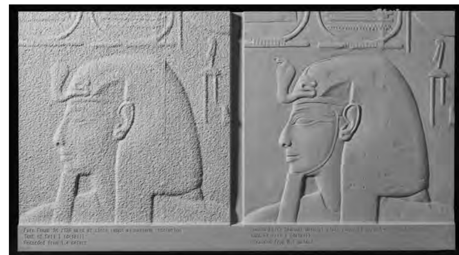
Maximum resolution recorded with the Faro scanner working at its minimum distance (left image) and the same section of the tomb of Seti I recorded with a Lucida scanner under normal working conditions (right image).
