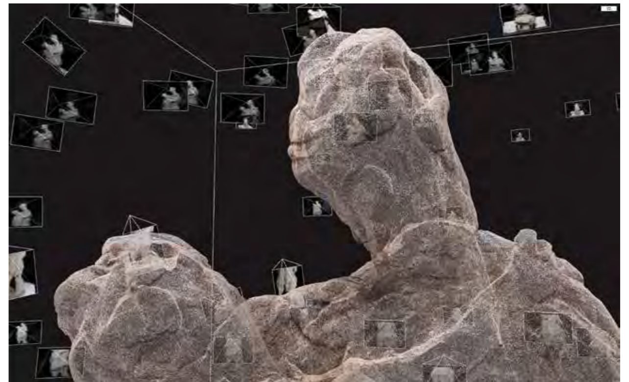
X. The point cloud up-close. Each individual point in the image above represents a common pixel found in more than one image (Screengrab from within RealityCapture)
