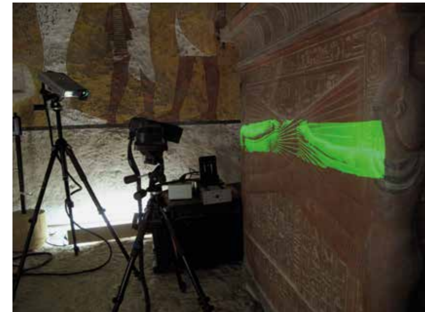
The Sidio White Light scanning system recording the surface of the sarcophagus of Tutankhamun. Photo by G. Dupond, courtesy of Factum Arte.
