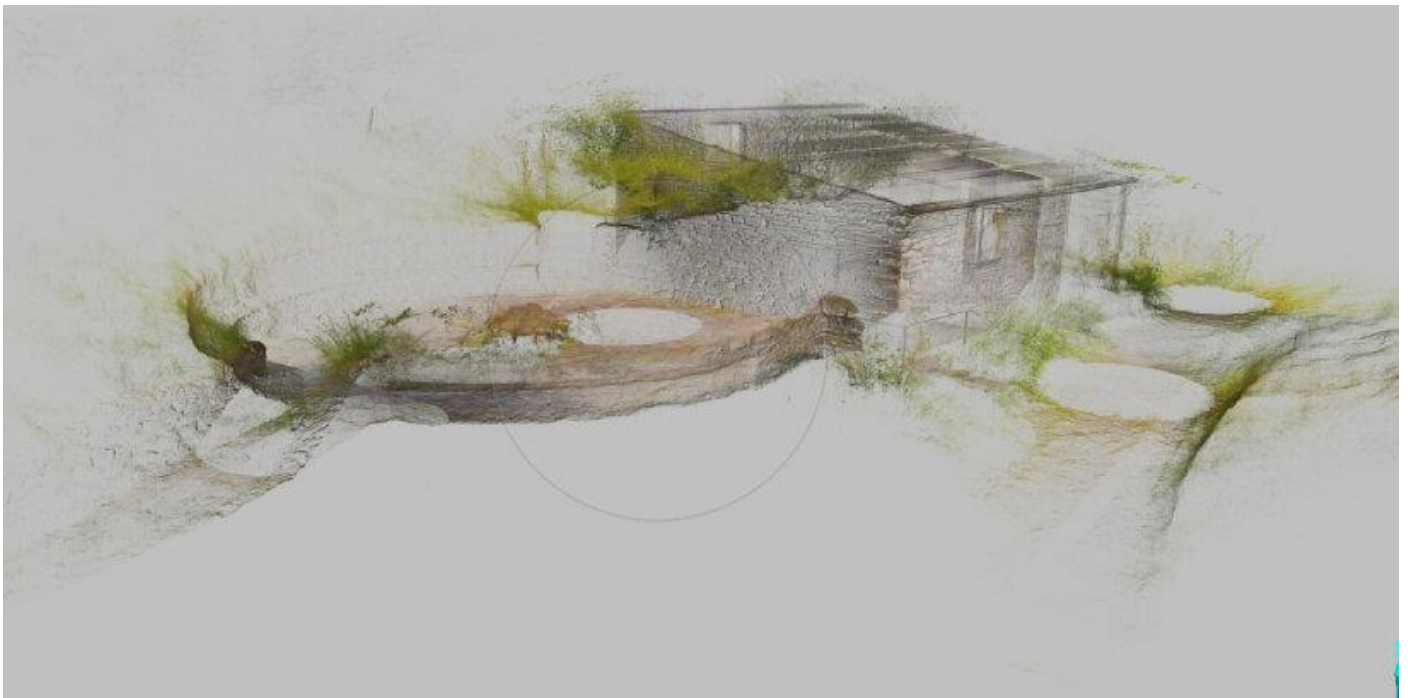
point cloud of the exterior of the Merz Barn following a first photogrammetry survey | image © Factum Foundation
