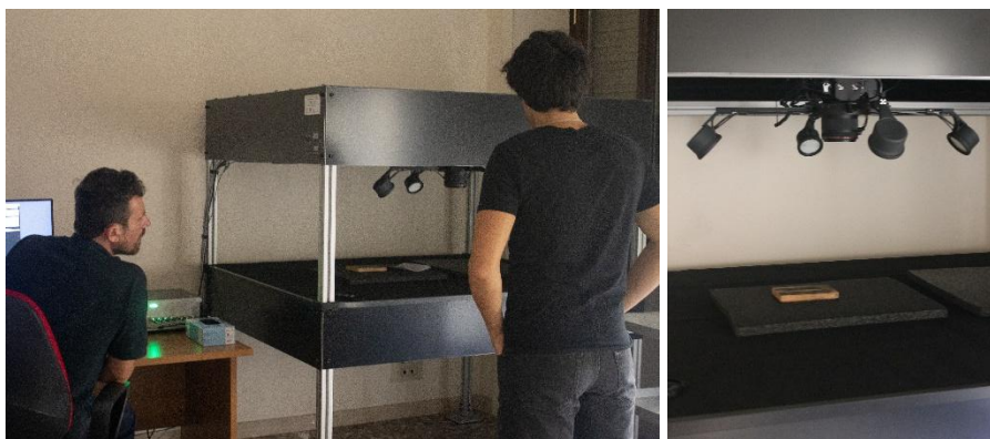
The Selene Photometric Stereo System © Factum Foundation
