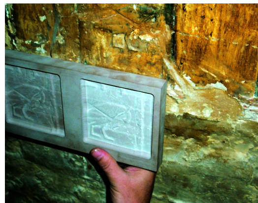
Left: One of the first routed samples in comparison with the original.
