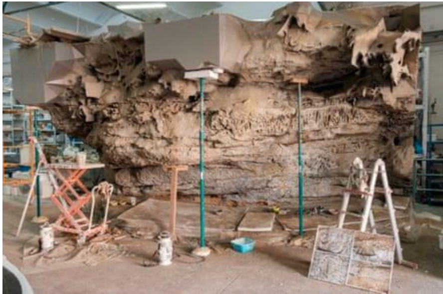
Sections of the cave replica, which is made out of resin-coated polystyrene and polyurethane, at Factum's workshop in Madrid. Photograph: Oak Taylor Smith/Factum Foundation
