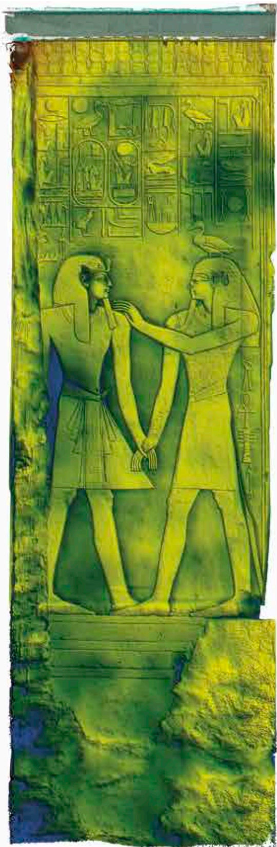
Depth maps of the pillars in Room J produced with 'Global Mapper' software.
