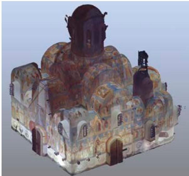
Clockwise from top: recording the cathedral using LiDAR; plans extracted from LiDAR data showing sections for panoramic photography recording; LiDAR model showing the internal fresco scheme.
