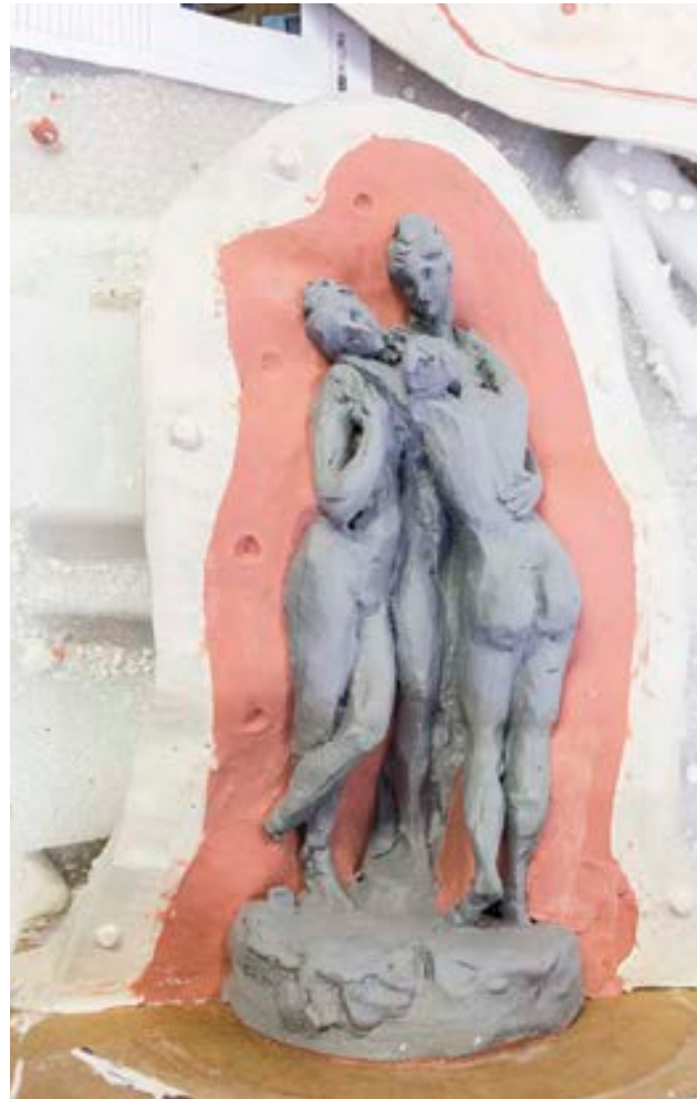
Creating a silicon mould from the 3D print of the Three Graces .
