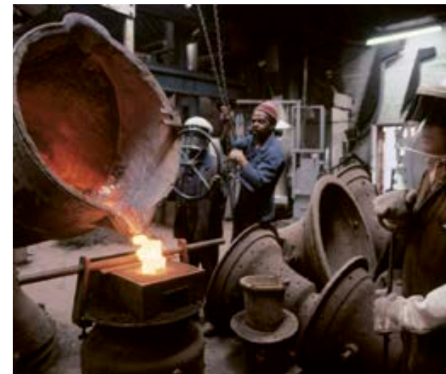
Casting bells at Whitechapel in 1997 with the traditional loam and greensand method.
