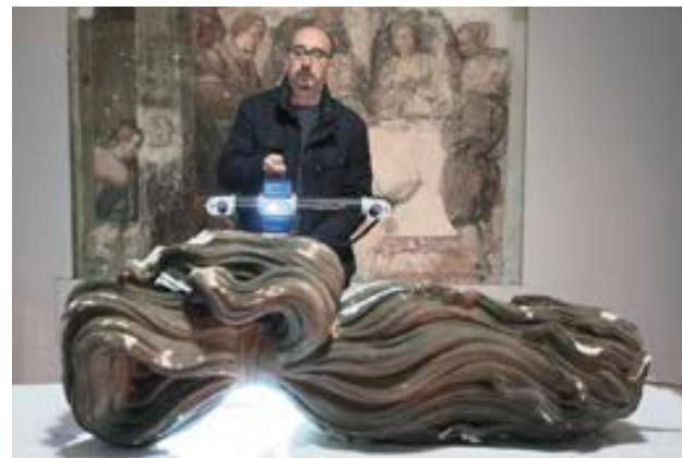
Recording Canova’s statue of a horse using a Breuckmann structured light scanner.
