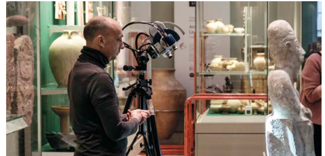
Recording Idrimi at the British Museum using a white-light scanner.
