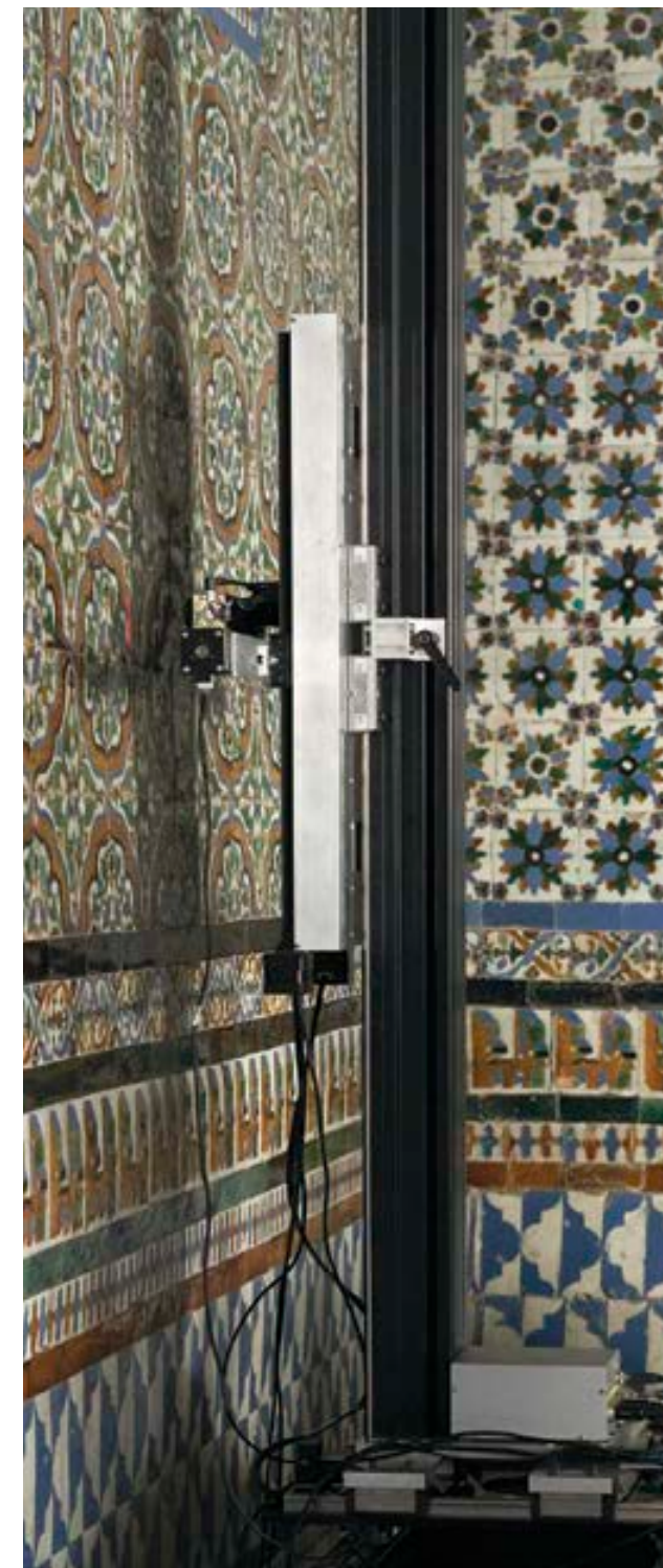
The Lucida 3D Scanner recording the azulejos of Casa de Pilatos in Seville.
