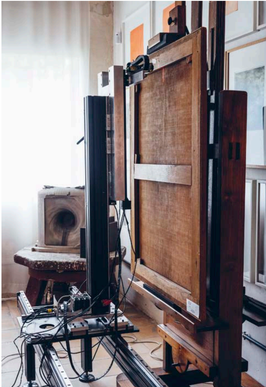
The Lucida 3D Scanner recording the back of the Ecce Homo , Caravaggio, 1604.
