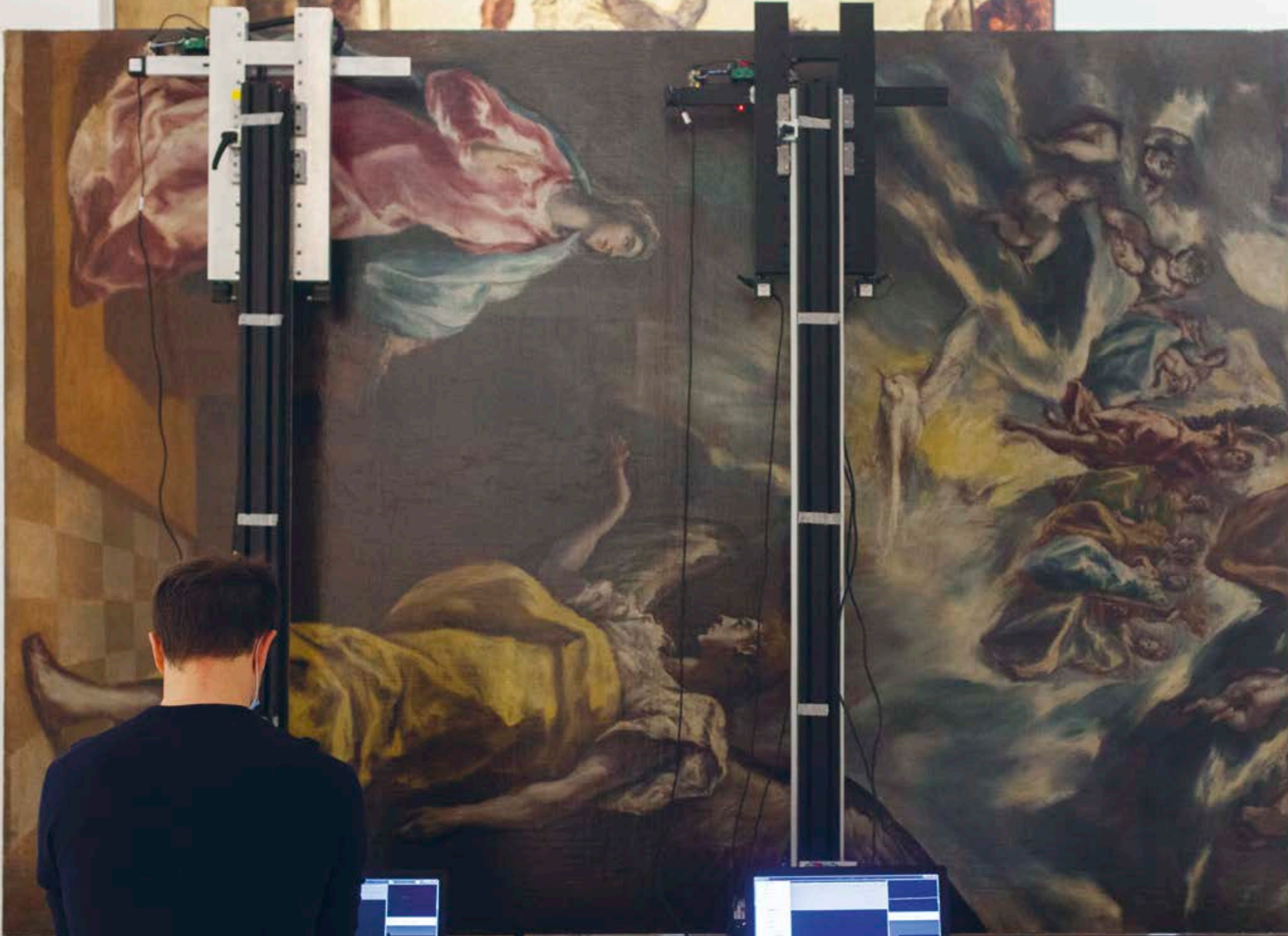
Two Lucida 3D scanners recording the surface of El Greco's Annunciation in the collection of Banco Santander, 2020.
