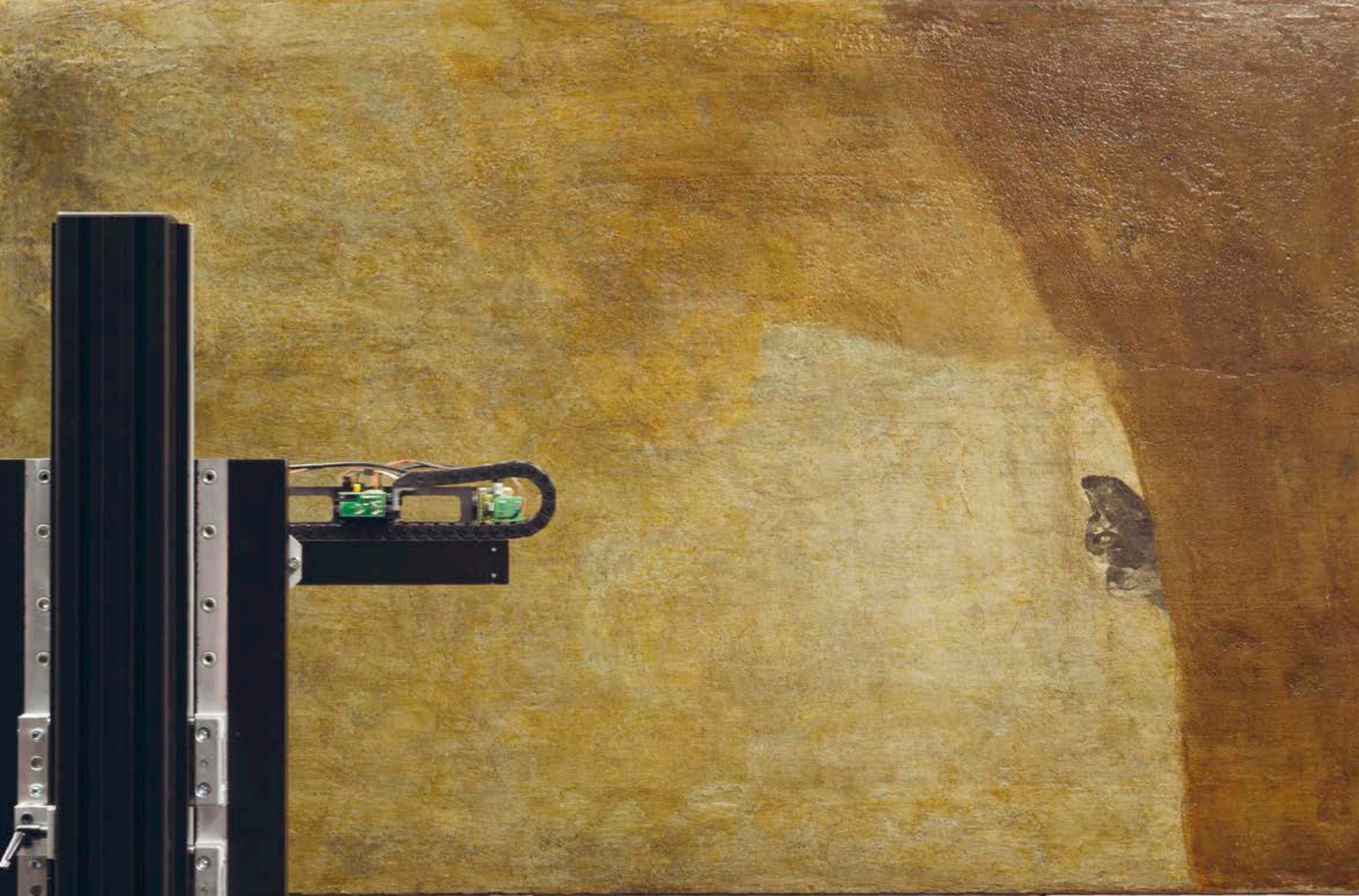
The Lucida 3D Scanner recording the surface of Goya's The Drowning Dog at the Museo del Prado, 2014.
