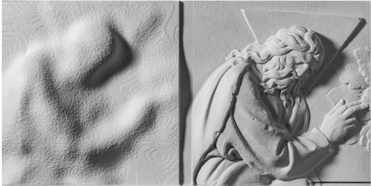
Image 2: CNC carved data from a FARO Focus 3DX 330 scanner a LiDAR scanner (left image) and same section of the façade of the Church of San Petronio recorded with a Nub3DWhite Light scanner (right image)
