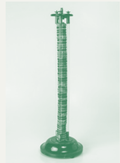
A Voltaic Pile, made by Aapps, London 1860s, Image: Oak Taylor-Smith
