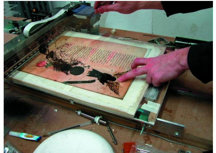
The vellum is positioned on the bed of the printer using a system of pin registered acetate sheets printed with outlines as a guide..
