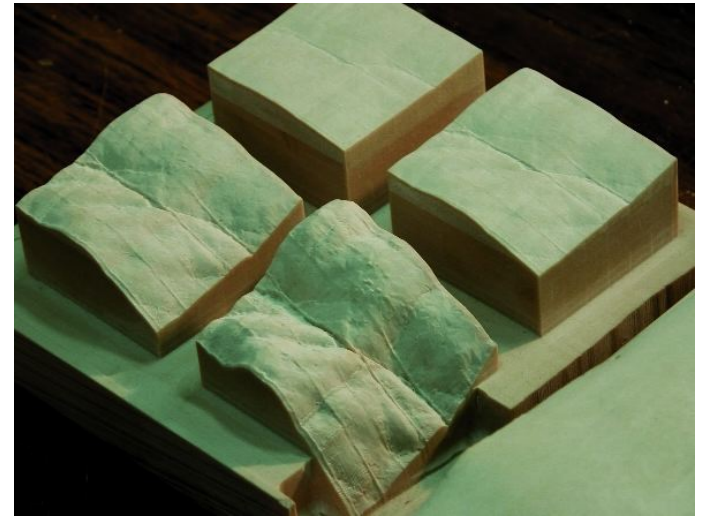
Routing tests with varying degrees of distortion to the Z axis to exaggerate the relief. The surface is very subtle and the exaggerated Z axis facilitates a detailed study of the superficial characteristics.
