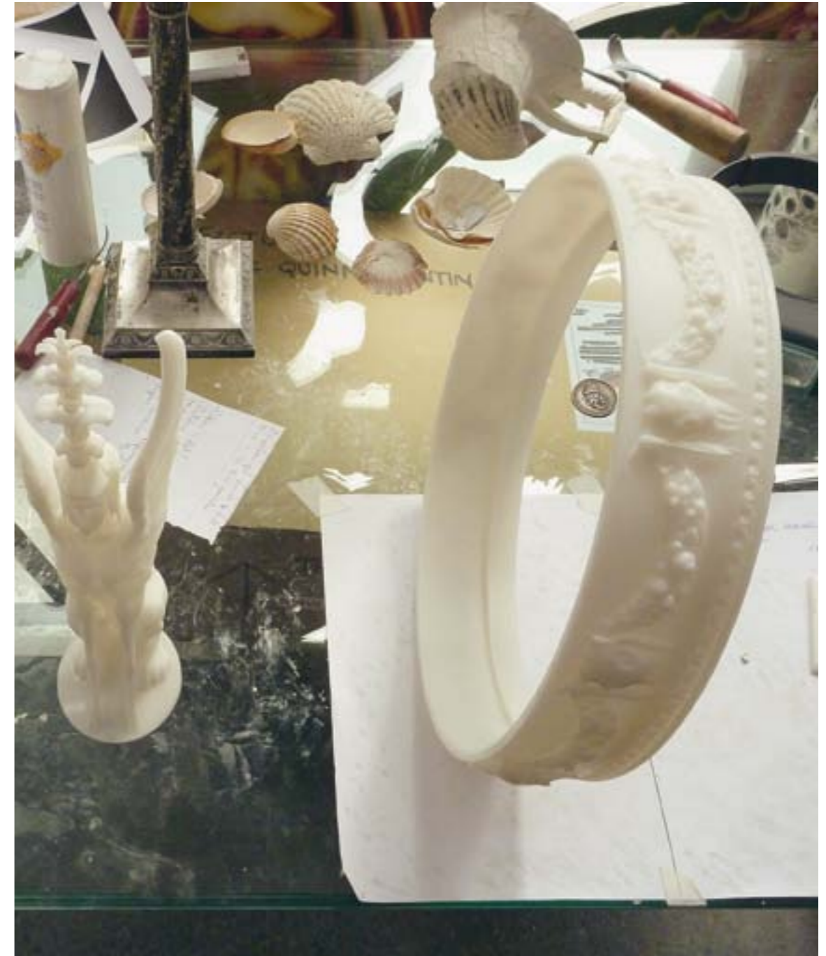
Stereolithographic prints of a sphinx/harpy and the crown from the top of the Isis tripod. Both elements were modelled in ZBrush and printed by Materialise in Lueven.
